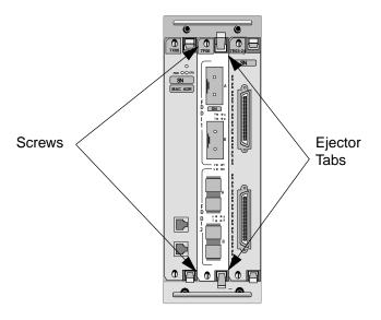
Figure 3-3. Removing the 7F06-02 Module from the 7C03 MMAC SmartSwitch
